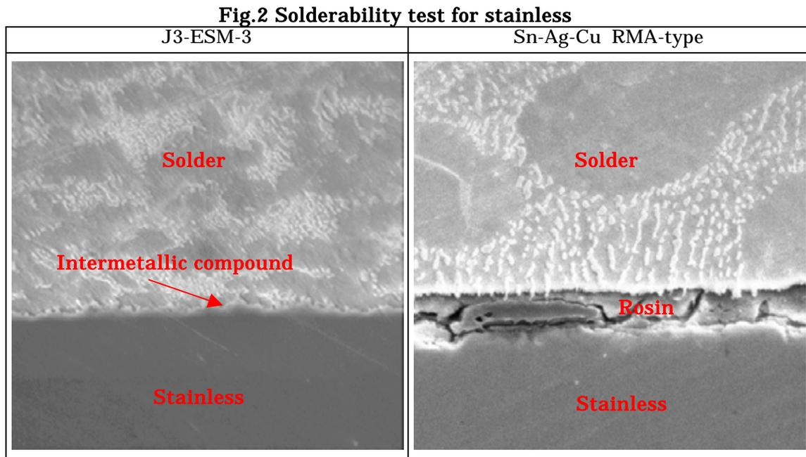
In the case of J3-ESM-3, which uses a fluorine activator, it can be observed that an intermetallic compound is formed between the stainless and the solder.
